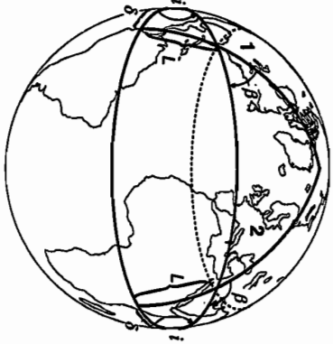
Fig. 6-12 Launch Window Geometry for Launches near the Ascending Node (1) and Descending Node (2). The angles shown are the orbital inclination ( i ), launch site latitude ( L ), and launch azimuth ( \beta ).
